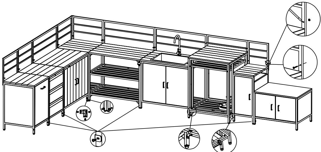
Disassemble the pre-installed screws on the legs, then use leg connection and the screws provided to fit each module at the front.
