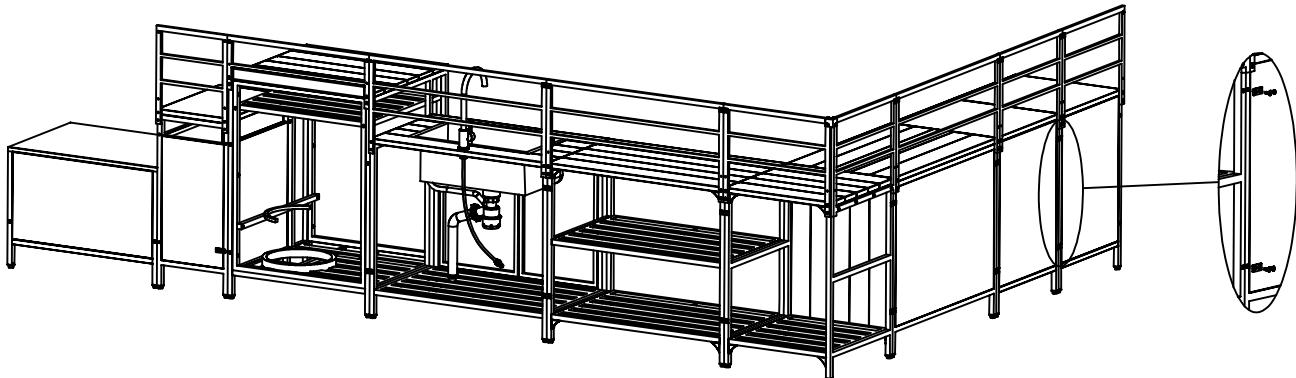
Disassemble the pre-installed screws on the modules, then use back connection and the screws provided to fit each module at the back.
