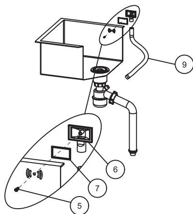
Connect the overflow pipe(9) to overflow head (5). Install overflow head to the sink with rectangle sealing ring (7) and M5x12 screw (5). Connect the other end of overflow (9) to part (13).
