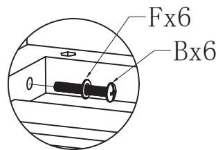
Attach the bottom panel (3) to the side panels with 6 pcs B screws and 6 pcs F screw washers.
