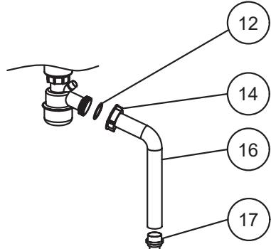
Install the drain pipe (16) to the drain pipe connector with sealing ring (12) and drain nut (14). Connect the water outlet (17) to drain pipe.
