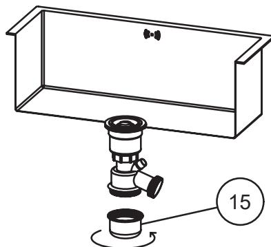
Install anti odor cup (15) onto grain cup connector (13).
