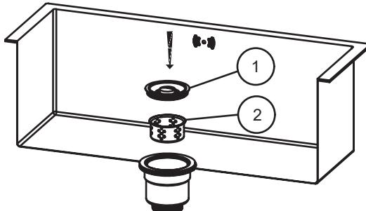
Put filter (2) and drain cup lid (1) onto drain cup (3).
