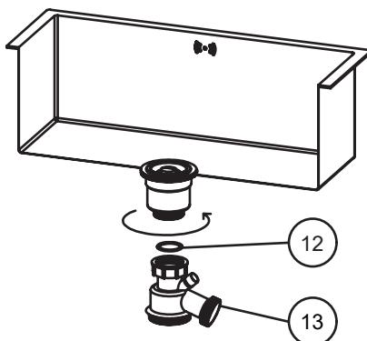
Put sealing ring (12) on part 4, install part 13.
