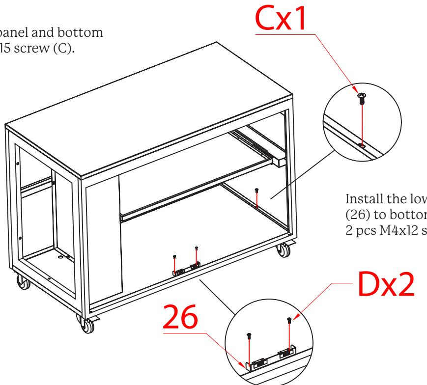
Install the lower magnet (26) to bottom panel with 2 pcs M4x12 screws (D).
