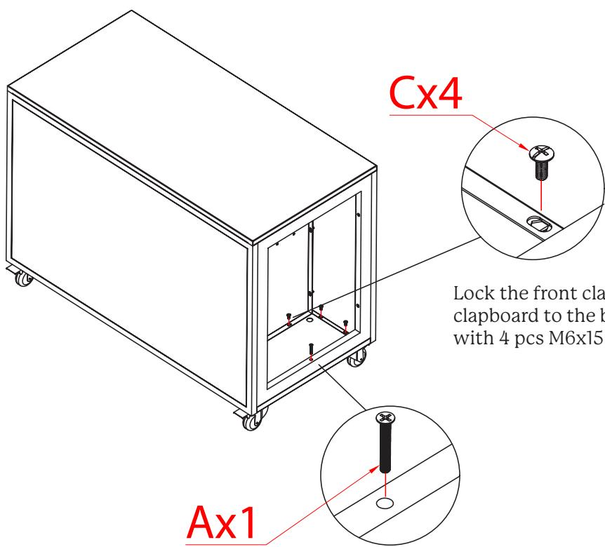
Lock the front clapboard and side clapboard to the bottom panel with 4 pcs M6x15 screws (C).
